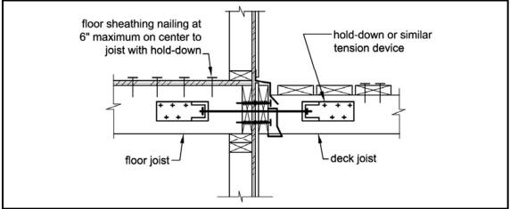
Does this detail belong as a minimum standard of deck construction now that the performance of a lag-screwed deck ledger is known to be quite sufficient?
